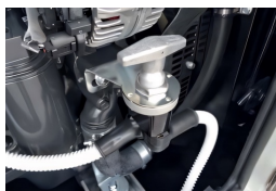
Batterieschalter Battery isolator switch
