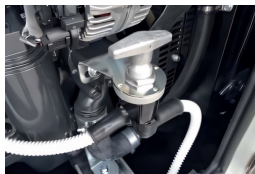
Batterieschalter Battery isolator switch
