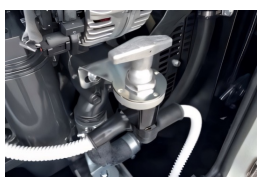
Batterieschalter Battery isolator switch
